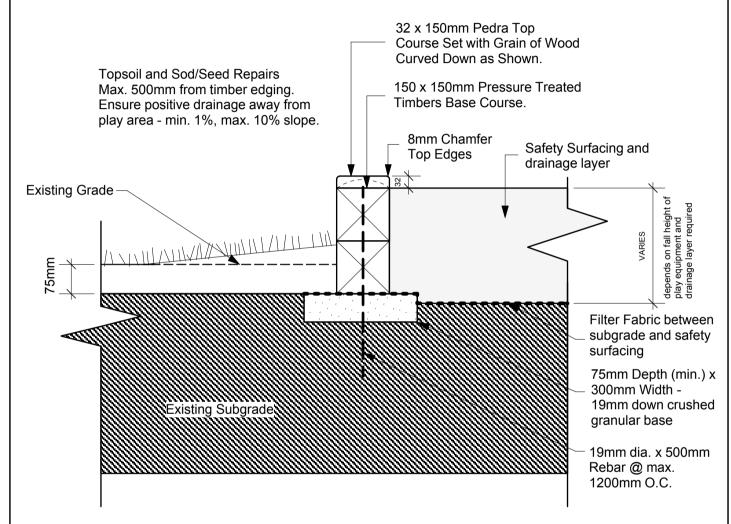
Base course timber shall be pinned with minimum of two (2) 19mm dia. rebar @ max. 1200mm O.C. Pedra top course shall be pre-drilled and screwed down using screws treated for ACQ use and sized to suit. Two parallel screws every 600mm O.C. along length and at ends. Only use but joints for straight sections of pedra. Min. length of timbers to be 1200mm. Install longest lengths possible.
